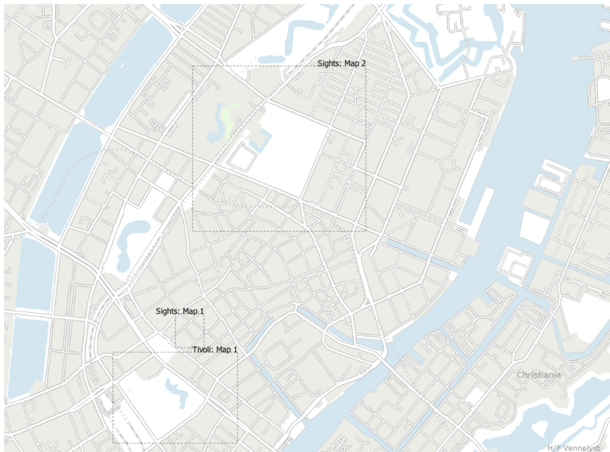
Рис. 11.10: Example of layout extents displayed in a QGIS project with two print layouts. The print layout named „Sights“ contains two map items, while the other print layout contains one map item.
