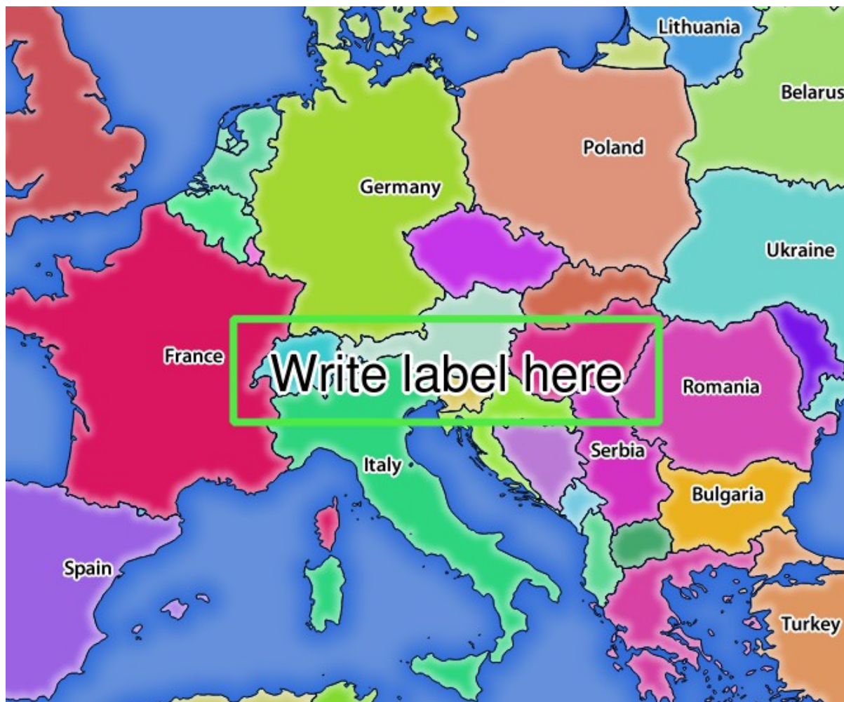
Рис. 17.9: Server response to a GetMap request with redlining parameters
