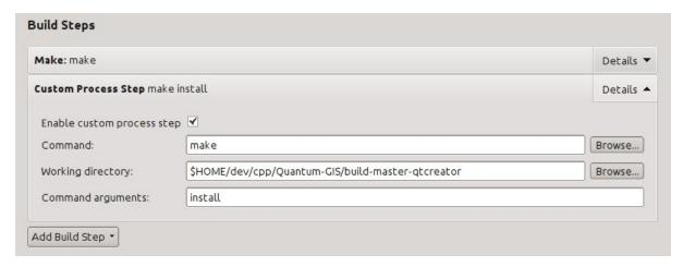
You are almost ready to build. Just one note: QtCreator will need write permissions on the install prefix. By default (which I am using here) QGIS is going to get installed to /usr/local/. For my purposes on my development machine, I just gave myself write permissions to the /usr/local directory.
