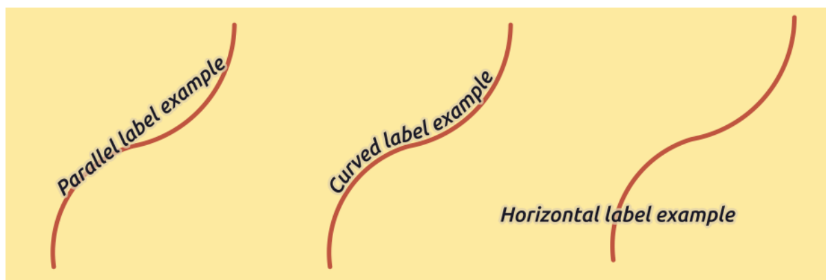
Figure 13.34: Label placement examples in lines
